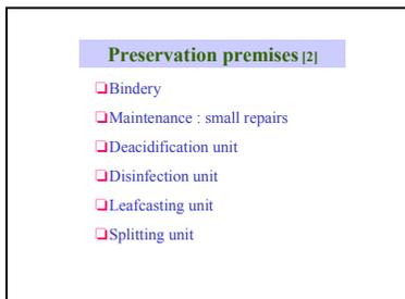
maintenance rooms for small repairs, binding section, deacidification plant, disinfection unit, mass treatment areas (with splitting or leafcasting machines), a documentation unit with preservation literature, and a training center...When designing the conservation lab it is important to separate humid areas with water sinks from other dry or dusting areas for instance.
