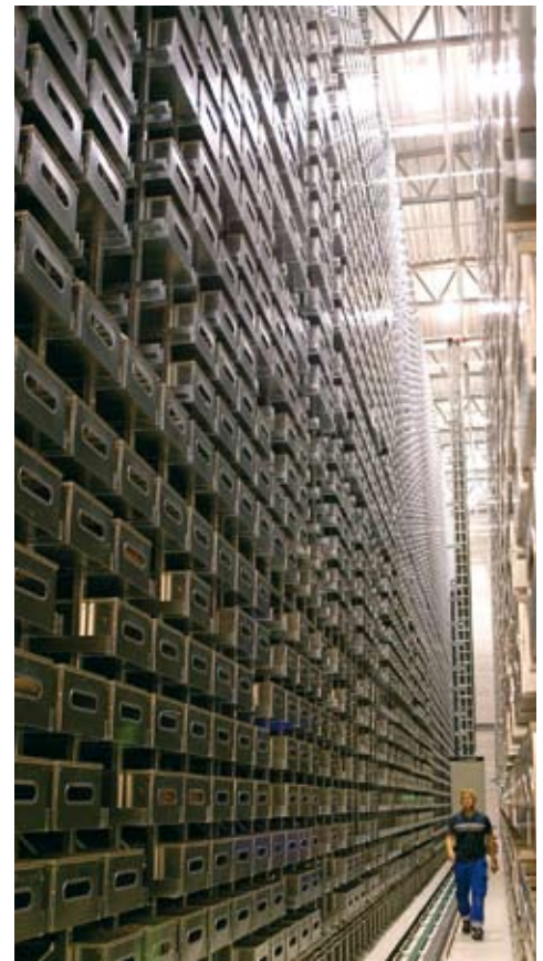
Modernity meets tradition. The National library in Mo in Rana contains a Repository Library with a world-class Automatic Storage Retrieval System (ASRS) with a capacity of 1,5 million items. Photo: Kjell Sommerseth
