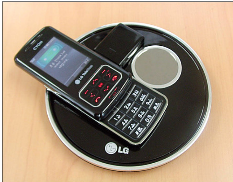
Figure 6. The Mobile Phone for the Print-Disabled and the NFC-Bluetooth Dongle
