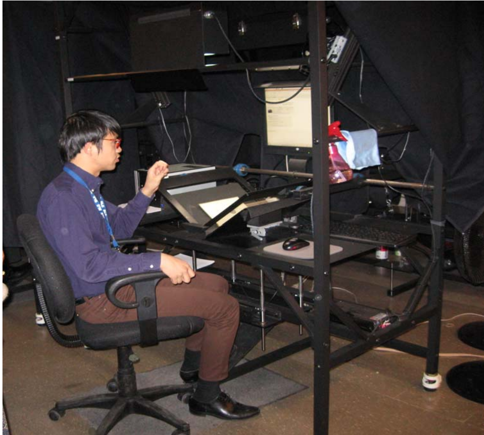
Figure 4: One of the Internet Archive scanning stations at the Boston Public Library.
